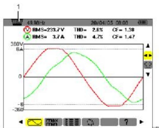
Figure 41: If the image memory is full, an attempted screen grab using the key displays the wastebasket icon (item 1).
