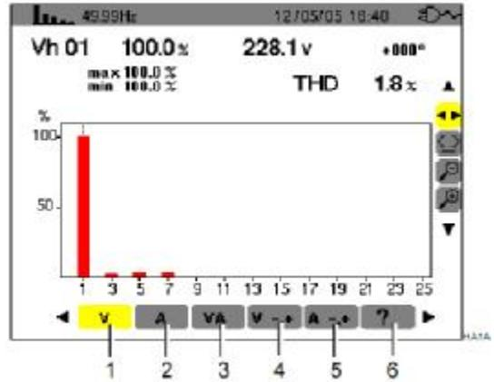
Figure 34: Example of display of Harmonics.
