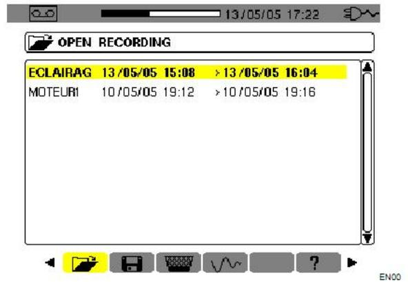
Figure 50: Example of recording campaigns screen.
