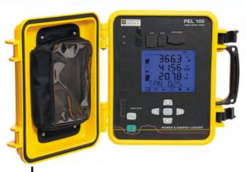
Large backlit screen with triple display & backlit symbol indicating the measurements in progress
