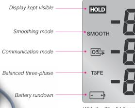
With the 73 x 54.3 mm LCD display, the user knows what the situation is at a glance. The battery rundown indicator light warns him when the period of autonomy is down to one hour
