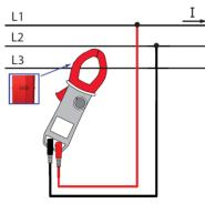
**Remark**: You can also measure the three-phase power on a balanced 4-wire network by proceeding in the same way, or by proceeding as for the measurement on a single-phase network, then multiplying the value found by three.
