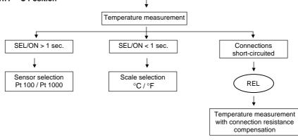
°C/°F selection and Pt 100 / Pt 1000 selection are saved in non-volatile memory. Pt 100 selection is indicated by display of  $\Omega$  symbol and Pt 1000 by display of k $\Omega$  symbol.
